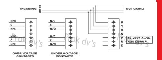
NOTE: FOR SHUNT RELEASE CONNECT C & N/O CONTACTS
